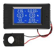
This product is an all in one instrument that can display Voltage, Current, Watts, Frequency, Power Factor and Wattage in WH. It can also record power consumption over a designated time period and sound internal alarm when it detects overload on the circuit.
